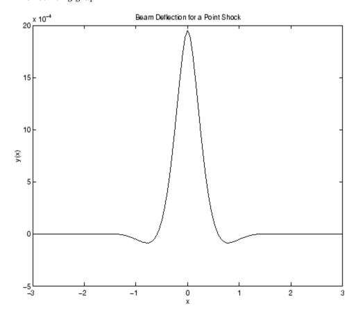
shows that the impact of a blow on a beam is highly localized; the greatest deflection occurs at the point of impact and falls off sharply from there.
