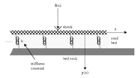
The shock could be induced by a pneumatic hammer blow.
