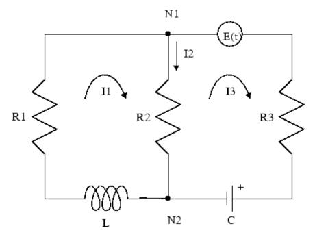
Let Rj and Ij, j = 1, 2, 3 be resistances (measured in ohms) and currents (amperes), respectively; L be inductance (henrys), and C be capacitance (farads); E(t) be the electromotive force, and Q(t) be the charge.
